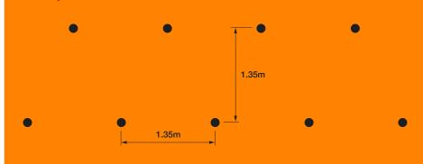
At the tops of walls and under gables, the topmost injection holes should not be more than 350mm below the upper edges of the cavity to be filled. Additionally under horizontal boundaries, for example under eaves windows or lintels, the centres between the topmost injection holes should not exceed 1.0m.
