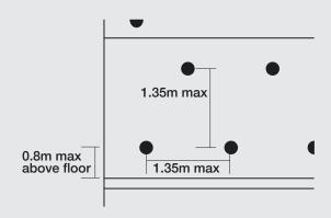
The second row of drill holes should be no more than 1.35m above the first row.
