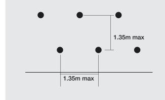
At the top of walls the topmost injection holes should not be more than 350mm below the roofline.
