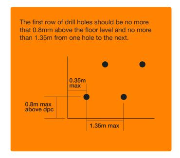
The drill pattern should be repeated at first floor and in each successive storey if applicable.
