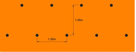
At the tops of walls and under gables, the topmost injection holes should not be more than 350mm below the upper edges of the cavity to be filled. Additionally under horizontal boundaries, for example under eaves windows or lintels, the centres between the topmost holes should not exceed 0.8m.
