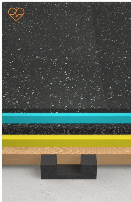
Cardio zones require floor systems to isolate the accumulative low frequency vibration created by multiple treadmill and spinning bike activities. The **ISO-Flex** Cardio systems isolate this vibration, preventing low frequency sound transmitting through the structure.
