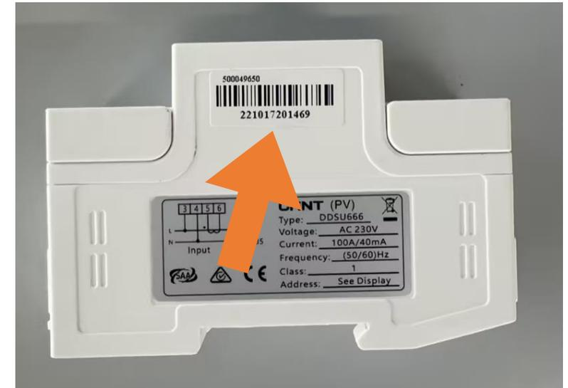
Tap the “Meter Location” to configure the grid side meter. The serial number (SN) can be entered manually or identified by scanning the bar code. If the GEN port is connected to the inverter or generator, the PV side meter also needs to be configured.
