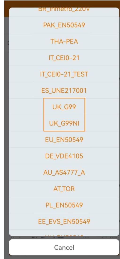
Tap the “ESS Safety Config” to check the relevant parameters of grid protection profile and power quality response mode and choose the corresponding grid code. We classify the installer account and user account through authority management, and the installer can modify grid protection and power quality response mode parameters.
