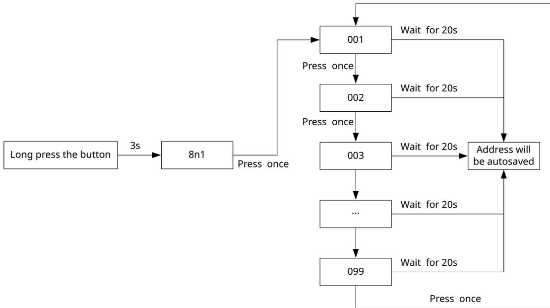
Figure 2-4 Communication address and baud rate setting diagram
