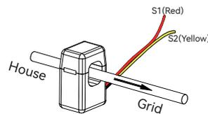
The direction of the arrow is consistent with the direction of the arrow inside the CT.
