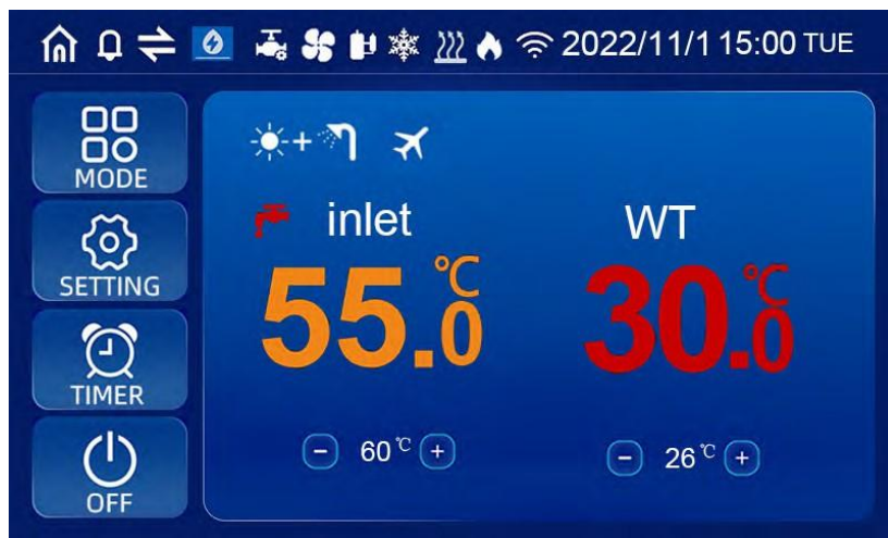
Dual mode display - left shows flow temp, right shows cylinder temp
