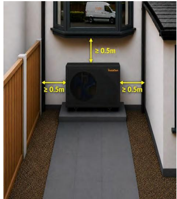
Recommended installation clearances around the unit
